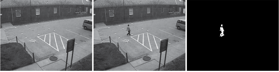
Fig. 1. Background subtraction results for the static unimodal Gaussian model. Left: static background image. Middle: image with human. Right: background subtraction results using the method in (2.4)
