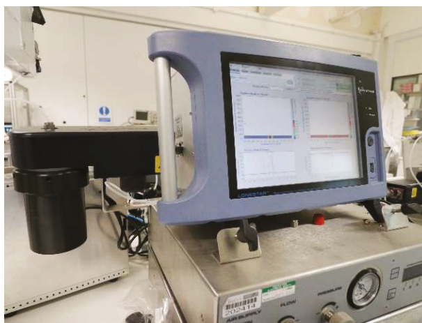
Figure 1. Field-asymmetric ion mobility spectrometer (FAIMS) setup.
