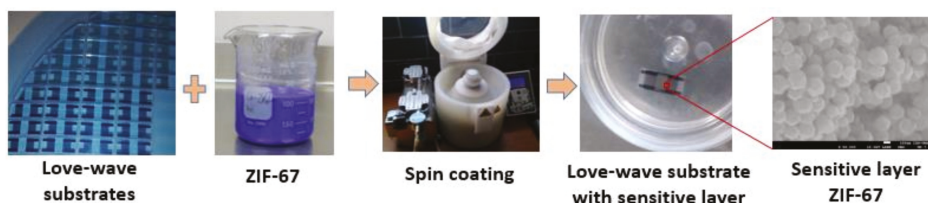
Figure 3. Process sequence of sensitive layer deposition on LW devices using the spin coating technique.
