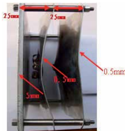
Fig. 27. Experimental result of flyer impact multi-layer structure
