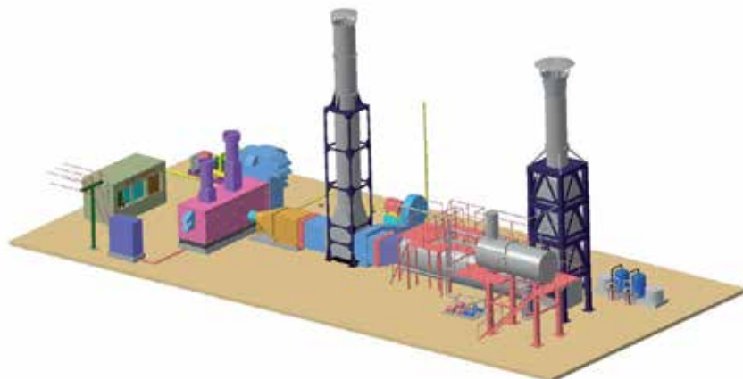
Figure 14. Model of an aeroderivative gas turbine cogeneration plant operating on natural gas and landfill gas
