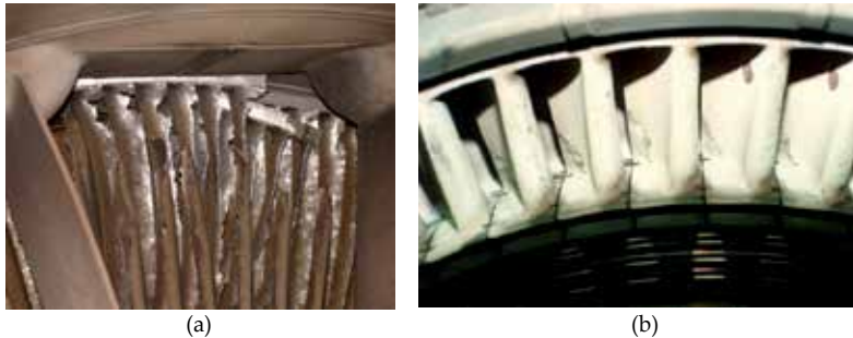
Figure 1. (a) FOD effects, (b) Turbine nozzles with deposits.
