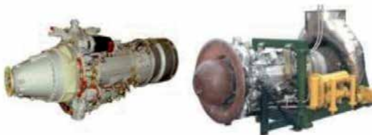
Figure 1. AI 20 turboprop (left) and AI 20 GM gas turbine (right) [2]
