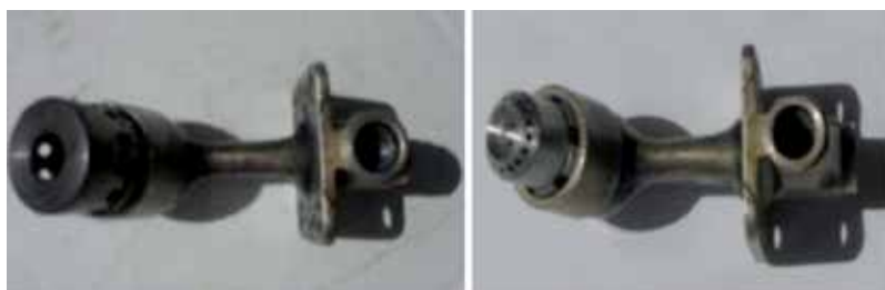
Figure 9. Injectors for liquid fuel for TV2-117A (left) and landfill gas for TA2 bio (right) [2]
