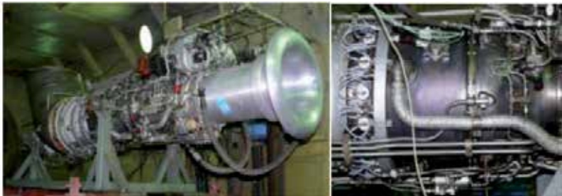
Figure 7. TV2-117A gas turbine (left) with detailed combustion chamber area (right)
