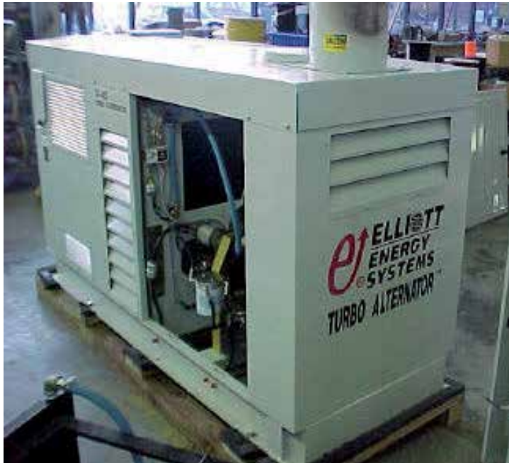
Figure 1. Elliott Energy Systems Microturbine, TA-45 model.
