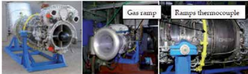
Figure 10. TA2 gas turbine (left) and TA2 bio gas turbine in the test cell (centre, right)
