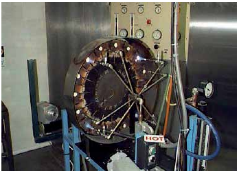
Figure 9. Wide JETS setup with four heating and cooling station [68].
