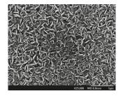
Figure 3. Field emission-scanning electron microscopy image of the APCVD tungsten doped VO<sub>2</sub> coating.
