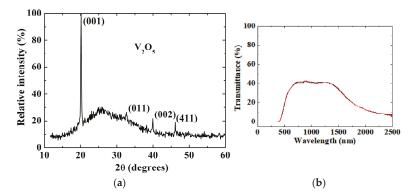
**Figure 6.** (a) X-ray diffraction of APCVD  $V_2O_5$  grown on F-doped SnO<sub>2</sub>. (b) No change in transmittance spectra observed over the region 250–2500 nm below  $T_c$  at 25 °C (black colour) and above  $T_c$  at 90 °C (red colour).
