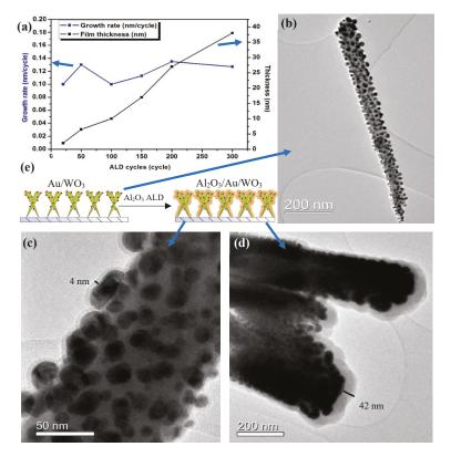
**Figure 8.** (a) Al<sub>2</sub>O<sub>3</sub> film growth rate (blue) and film thickness (black) as a function of reaction cycles, (b) Au/WO<sub>3</sub> structure, (c) Au/WO<sub>3</sub> with 50 cycles ALD Al<sub>2</sub>O<sub>3</sub> growth on top, (d) Au/WO<sub>3</sub> with 300 cycles ALD Al<sub>2</sub>O<sub>3</sub> growth on top, (e) Schematic procedure of ALD Al<sub>2</sub>O<sub>3</sub> growth.
