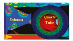
**Figure 7.** Simulation of transport species within the components of the APCVD reactor. The simulation showed an increase of the fluid's velocity from  $2.359 \times 10^{-3}$  m s<sup>-1</sup> to  $3.283 \times 10^{-3}$  m s<sup>-1</sup>, i.e., an increase of velocity of 39.18% due to temperature change. (Image courtesy of Delta Nano—Engineering Solutions Ltd., London, UK).
