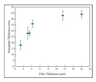
Figure 11. Variation of nanoplate thickness with film thickness.
