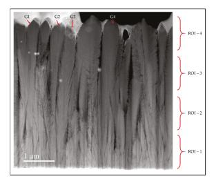
Figure 13. Cross-section STEM image of sample G prepared via pp-MOCVD.
