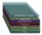
**Figure 4.** Schematic diagram of the semitransparent PSC using the graphene as top electrode. Reproduced with permission from reference [105].
