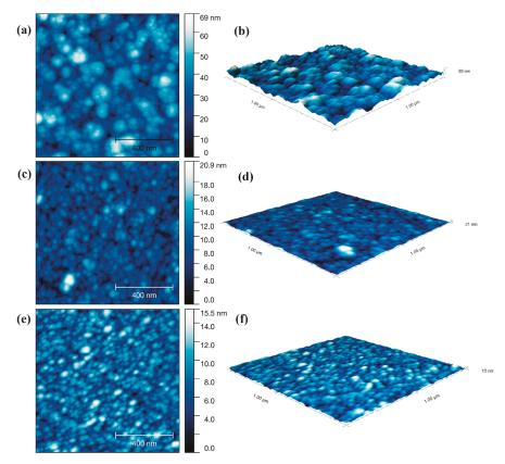
**Figure 4.** AFM scans and 3D images of Al<sub>2</sub>O<sub>3</sub> films deposited at 350°C via (**a**,**b**) continuous CVD; (**c**,**d**) pulsed CVD (1 min ATSB pulse) and (**e**,**f**) pulsed CVD (20 s ATSB pulse).
