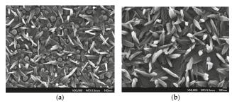
Figure 4. Field emission-scanning electron microscopy images of APCVD vanadium oxides using oxygen flow rate of 0.4 (a) and 0.8 L min<sup>-1</sup> (b).
