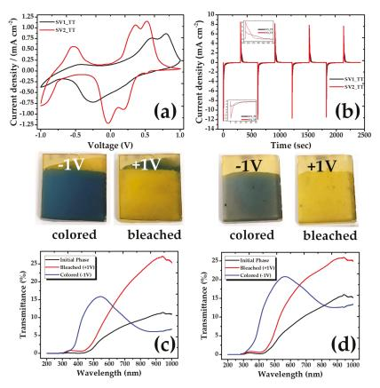
**Figure 4.** (a) Cyclic voltammograms after annealing, (b) Chronoamperometry after annealing, (c,d) UV-Vis transmittance comparison of the initial, bleached and colored state of the V<sub>2</sub>O<sub>5</sub> coatings, (c) SV1\_TT, (d) SV2\_TT.
