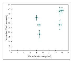
Figure 12. Variation of nanoplate thickness with mean film growth-rate.
