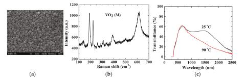
Figure 5. Field emission-scanning electron microscopy image (a) and (b) Raman spectroscopy of APCVD VO<sub>2</sub> grown on SnO<sub>2</sub>-precoated glass substrates. (c) Transmittance spectra below  $T_c$  at 25 °C and above  $T_c$  at 90 °C over the region of 250–2500 nm to study the thermochromic performance.
