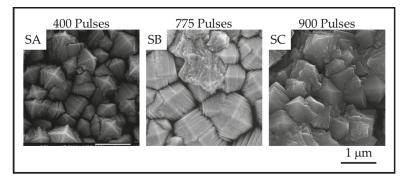
Figure 6. Plan-View SEM images showing the surface of anatase crystals for  $TiO_2$  samples on stainless steel prepared with SA. 400 pulses; SB. 735 pulses and SC. 909 pulses.
