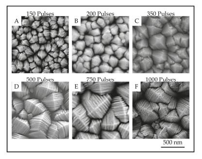
**Figure 5.** Plan-view SEM images showing the surface of anatase crystals for TiO<sub>2</sub> samples on fused silica prepared with (**A**). 150 pulses; (**B**). 200 pulses; (**C**). 350 pulses; (**D**). 500 pulses; (**E**). 750 pulses and (**F**). 1000 pulses.
