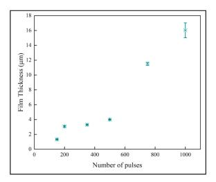
Figure 10. Sample thicknesses increases with number of pulses.
