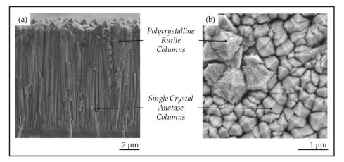
**Figure 2.** (a) Cross-section morphology on a fracture surface and (b) plan-view surface morphology of  $TiO_2$  films prepared by pulsed-pressure metalorganic chemical vapor deposition (pp-MOCVD).
