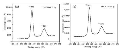
Figure 5. The XPS spectrum of Ti 1*p* states of (a) Ti-CNT #1 and (b) Ti-CNT #2.
