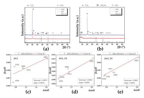
**Figure 2.** GIXRD patterns for (**a**) SV1 before and after annealing, (**b**) SV2 before and after annealing with red and blue line, respectively. In addition, GIXRD pattern corresponding to FTO was added (black line). (**c**–**e**) Williamson-Hall plots for SV1, SV1\_TT and SV2, respectively with corresponding values for intercept and slope as inset.
