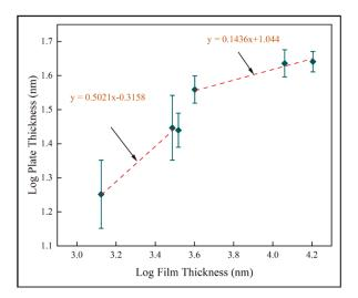
Figure 16. Log transformed plate thickness for mean data on fused silica substrates (samples A-F).
