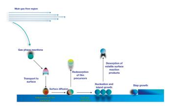
Figure 1. Schematic view of CVD (Chemical Vapour Deposition) process [1].
