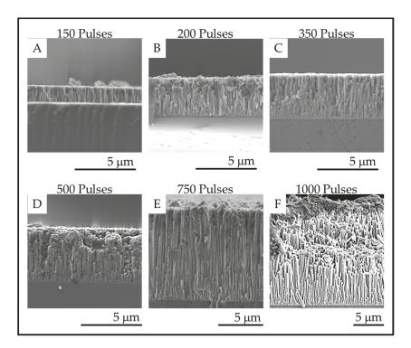
Figure 9. Fracture surface SEM images of the TiO<sub>2</sub> coatings deposited on fused silica with (A). 150 pulses; (B). 200 pulses; (C). 350 pulses; (D). 500 pulses; (E). 750 pulses and (F). 1000 pulses.
