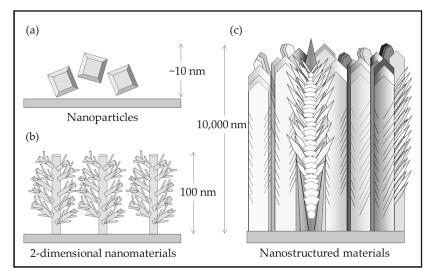
**Figure 1.** Illustration of (a)  $TiO_2$  nanoparticles; (b) rutile nanorods with secondary structures grown on a substrate [15]; (c) nanostructured  $TiO_2$  in a solid coating adhered to a substrate [14].
