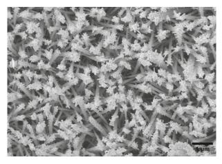
Figure 7. SEM image of Au/WO<sub>3</sub> film deposited via CVD (top view).
