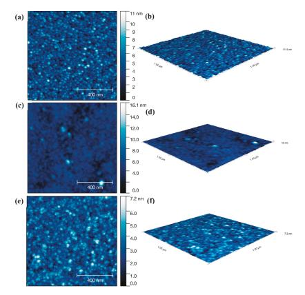
**Figure 6.** AFM scans and 3D images of  $Al_2O_3$  films after 250 ALD cycles, on (**a**,**b**) silicon; (**c**,**d**) quartz; (**e**,**f**) glass. A cycle includes 2.5 s ATSB pulse, 3 min Ar purge, 2 s H<sub>2</sub>O pulse and 3 min Ar purge, deposition temperature 200 °C, gas flow rate 120 sccm.
