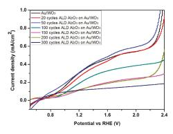
Figure 10. J-V curves of Al<sub>2</sub>O<sub>3</sub>/Au/WO<sub>3</sub> during photoelectrochemical measurement.
