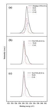
Figure 4. The XPS spectra of O 1s states of (a) pristine CNTs, (b) Ti-CNT #1, and (c) Ti-CNT #2.
