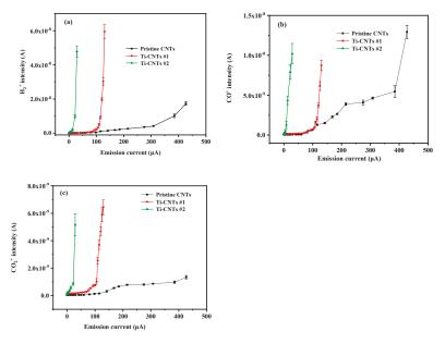
**Figure 11.** Gas desorption along with variation of FE current for pristine CNTs, CNTs #1 and CNTs #2. (a) H<sub>2</sub><sup>+</sup> intensity, (b) CO<sup>+</sup> intensity, (c) CO<sub>2</sub><sup>+</sup> intensity.
