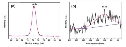
**Figure 2.** High resolution XPS spectra of (**a**) Al 2p and (**b**) Si 2p of Al<sub>2</sub>O<sub>3</sub> film deposited on glass via CVD.
