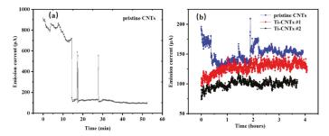
Figure 7. Emission current summary of Ti-coated CNTs and pristine CNTs over time. (a) Aging conditioning of pristine CNTs during a short period. (b) Stability comparison.
