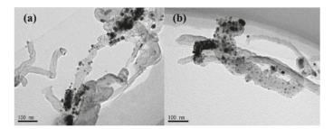
**Figure 2.** HRTEM of titanium-coated CNTs under the process of magnetron sputtering. (a) Ti–CNTs #1 with 40 s irradiation and 42 s DC sputtering. (b) Ti-CNTs #2 with 60 s irradiation and 42 s DC sputtering.
