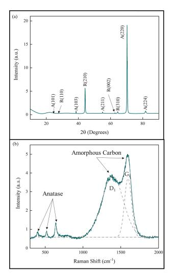
Figure 4. (a) XRD pattern and (b) Raman spectrum of TiO<sub>2</sub> coatings prepared by pp-MOCVD.
