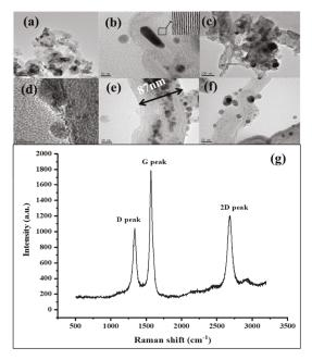
**Figure 1.** High-resolution transmission electron microscopy (HRTEM) images of (**a**) pristine MWNT, (**b**) magnification of single tube of pristine CNTs (inset: magnification of HRTEM image of outer shells.), (**c**) Ar<sup>+</sup>-irradiated MWNTs, (**d**) Ti nanoparticles on the normal outer wall of CNTs, (**e**) Ti nanoparticles on the larger-diameter defective CNTs, (**f**) Ti nanoparticles on the "junction" of defective CNTs, (**g**) Raman spectrum of pristine CNTs.
