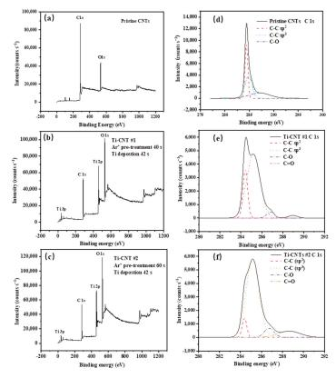
**Figure 3.** The XPS spectra of different CNT samples: (a) pristine CNTs, (b) Ti-CNTs #1, (c) Ti-CNTs #2, (d) C 1s states of Pristine CNTs, (e) C 1s states of Ti-CNTs #1, (f) C 1s states of Ti-CNTs #2.
