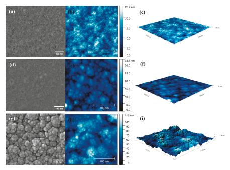
**Figure 3.** SEM images, AFM scans and 3D images of Al<sub>2</sub>O<sub>3</sub> films deposited for 24 h with 150 sccm Ar gas flow, precursor temperature at 120 °C and deposition temperature at (**a**–**c**) 300 °C; (**d**–**f**) 350 °C; (**g**–**i**) 400 °C.
