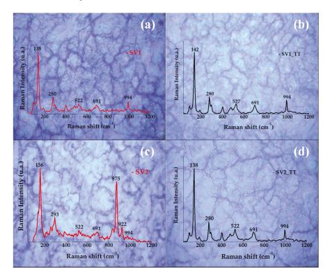
**Figure 3.** Raman spectra overlapped over optical microscopy images (100× magnification) of SV1 (20 mL, 0.02 M) and SV2 (20 mL, 0.01 M) samples, (**a**,**c**) before annealing, (**b**,**d**) after annealing.
