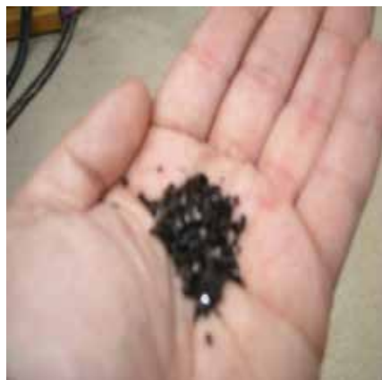
Photo 15. Water cooled slag in the form of granules
