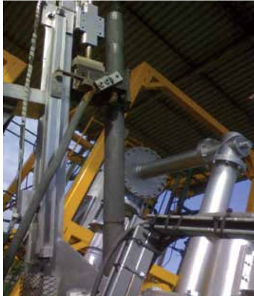
Photo 9. Movement Mechanism of the graphite electrode
