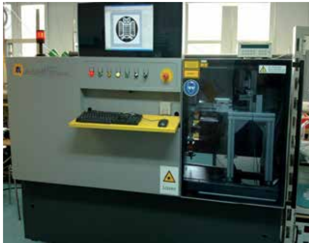
Figure 5. Prototypical CO 2 -laser sintering facility used for sintering and densification of green thin film ceramic layers.
