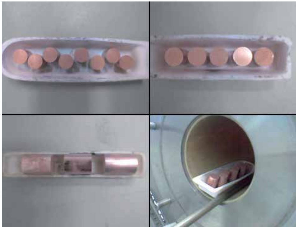
Figure 1. Ternary Cu-Ni alloys distributed in alumina boat for sintering and homogenizing heat treatment in vacuum furnace.
