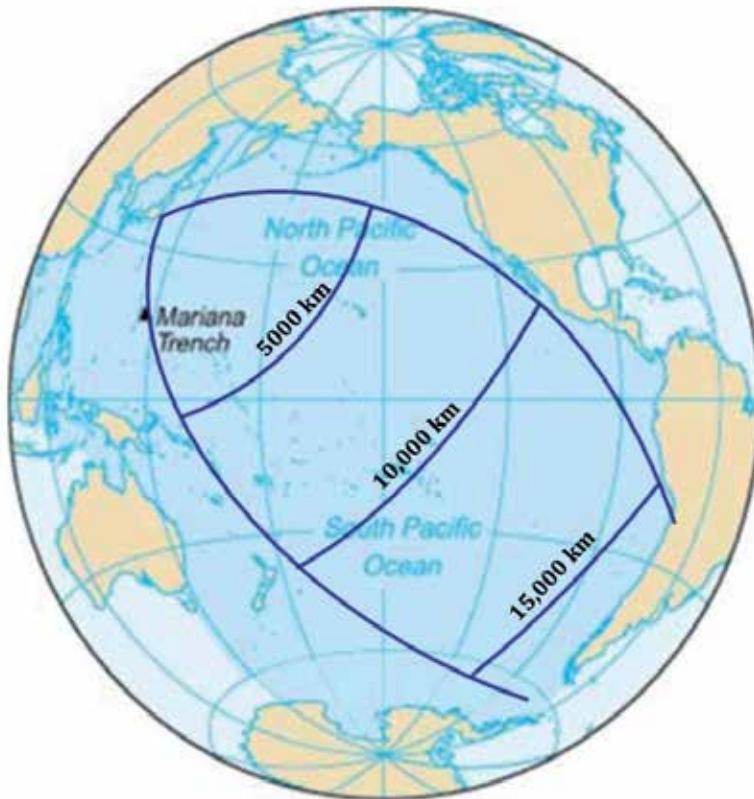
Figure 2. Propagation geometry of 2011 Japan tsunami in a lune of angle 90^\circ with wavefronts at intervals of 5,000 km
