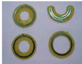
Fig. 36. The coupling antenna for the sensory system.
