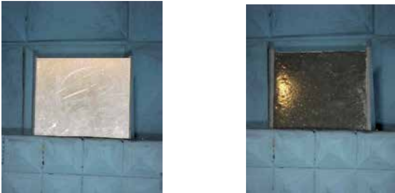
Fig. 11. Flat plate assembled in an anechoic chamber: metal face (left) and ERAM face (right).
