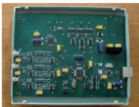
Fig. 27. Constructive realization of the block of the microcontroller and sensor of surplus pressure on the basis of PRMT
