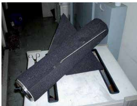
Fig. 26. View of the missile's section covered with ERAM.
