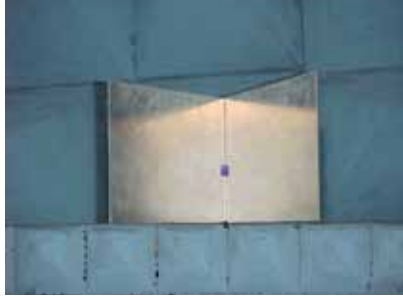
Fig. 14. Assembly of a dihedral on the azimuth positioner.
