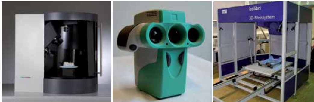
Fig. 1. Several fringe projection based measurement systems developed at Fraunhofer IOF: kolibri flex mini, kolibri CORDLESS, kolibri step (from left to right)
