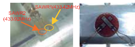
Fig. 30. The setup of the SAWRs and the strain gage on the shaft.
