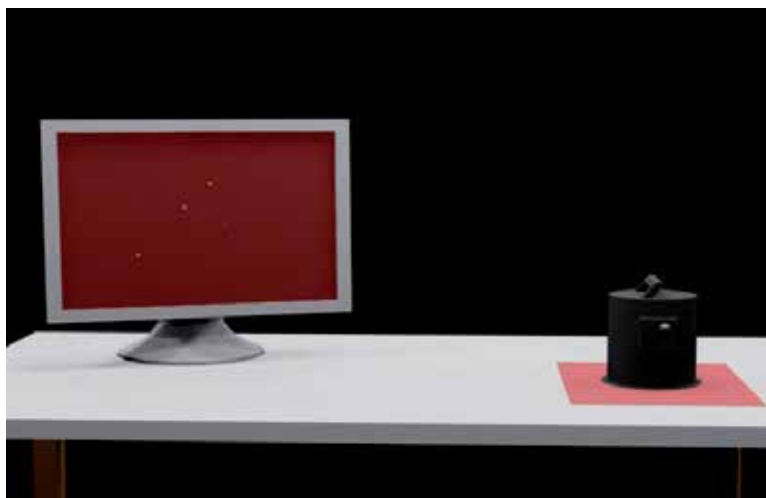
Fig. 5. Hand-held unit for internal use for fast recognition of UV, and IR pigments
