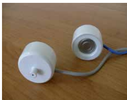
Fig. 27. Constructive realization of the block of the microcontroller and sensor of surplus pressure on the basis of PRMT
