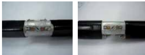
Fig. 35. The rotational shaft equipped with two SAWRs.
