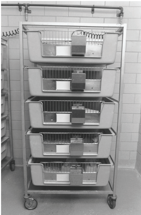
Fig. 12 Caging system for group housing guinea pigs composed of large, hard plastic and stainless steel cages, automatic watering system, stainless steel feeders, and cage card-holders.
