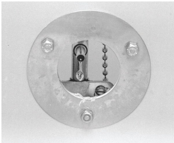
Fig. 14 Automatic watering device found in the back of a guinea pig cage. Note that the valve is located outside of the cage.
