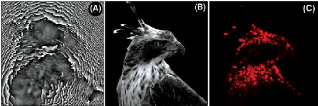
Fig. 16. Results obtained by a phase-only CGH for the same desired reconstruction of figure 13 (a) phase distribution of the CGH, designed using one hundred iterations of the IFTA for the desired image shown in Fig. 13a, (b) computer reconstruction, (c) optical reconstruction: a strong speckle noise is present. Reprinted with permission of SPIE (Neto, L. G., 2004).
