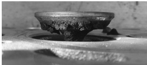
Figure 5. Soot present due to EGR on intake valve, cylinder two.
