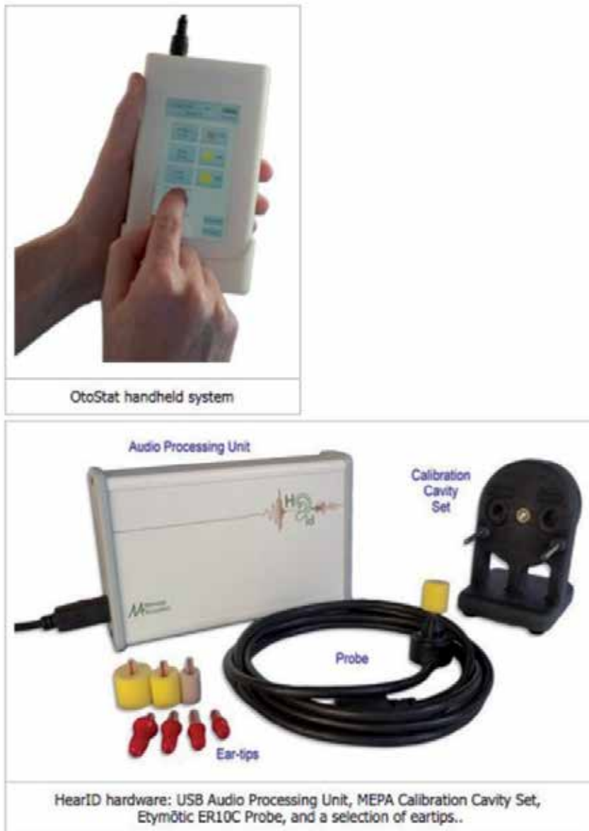
Figure 1. The Mimosa Acoustic devices capable of recording wideband reflectance and OAEs. Data from the Mimosa Acoustics website ( http://www.mimosaacoustics.com ).
