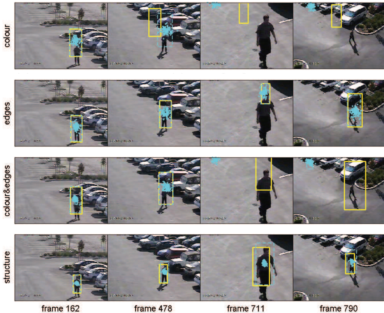
Fig. 3. Example video frames with average output of the tracking algorithm (solid line rectangle), a single trial output (dashed line rectangle and particles) superimposed, sequence man
