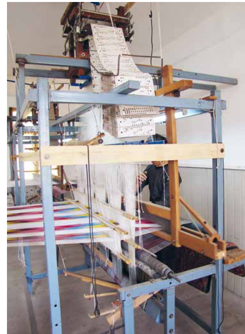
In the workshop of the weaver Fazletdin. Near Andijan in the Fergana Valley Fazletdin has developed his own combination of ikat weaving and the Jacquard technique.
