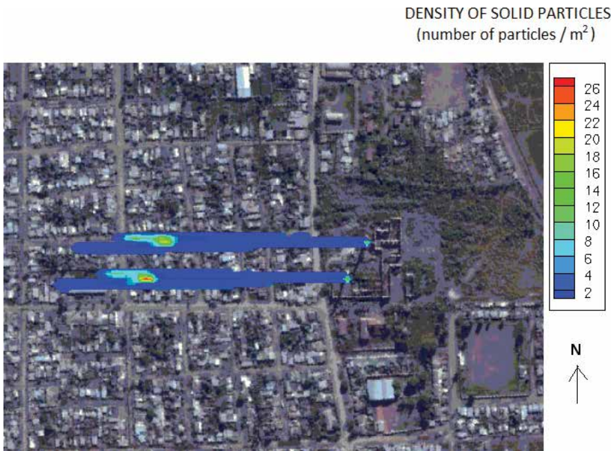
Figure 12. Copper concentration at ground level simulated with 10 \times 10 m grid mesh on a satellite image.
