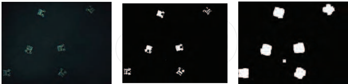
Fig. 3. An image captured by the system camera (left), the binary image obtained by the segmentation process (center) and the resulting binary image after applying two morphological operations (right)
