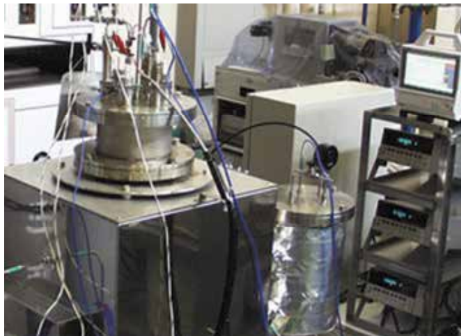
Fig. 9. Photo of the comparison apparatus of oxygen sensors. Three sensors can be compared in liquid LBE.
