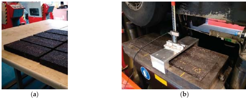
Figure 5. The rutting test: (a) the prepared slabs for testing and (b) the rut depth measuring procedure.
