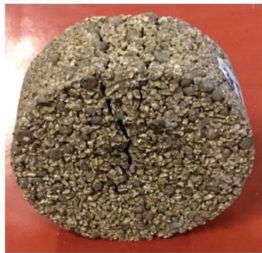
Figure 4. Gyratory sample with synthetic aggregates.
