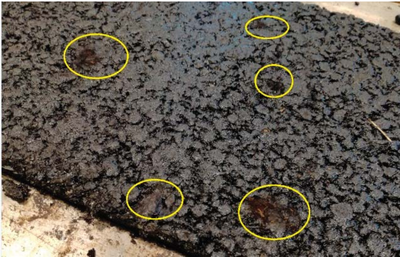
Figure 16. An example of an asphalt slab produced by the dry approach (mixing peat with aggregates in the asphalt mix).
