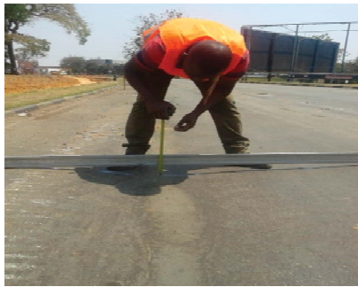
Figure 6. Profile measurements on Kitwe-Ndola Road.
