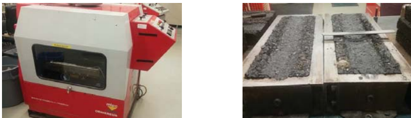
Figure 7. The French rutting test equipment.
