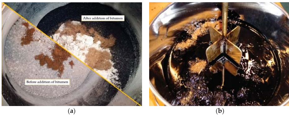
Figure 15. Mixing of peat fibers in the asphalt mix: (a) the first approach and (b) the second approach.
