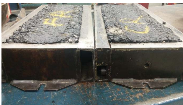
Figure 14. RAP mix slabs after rutting test.
