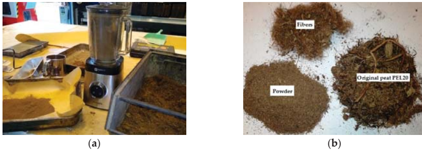
Figure 1. The preparation of peat material for testing: (a) grinding and (b) sieving.
