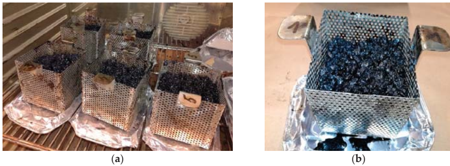
Figure 14. The drainage test: (a) asphalt mixes with peat and (b) the REF asphalt mix [24].
