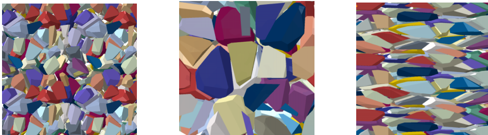
Figure 3.25: Examples of materials with particle reinforced matrix: statistically isotropic polyhedral particles, oblate particles, elongated particles (left to right)
