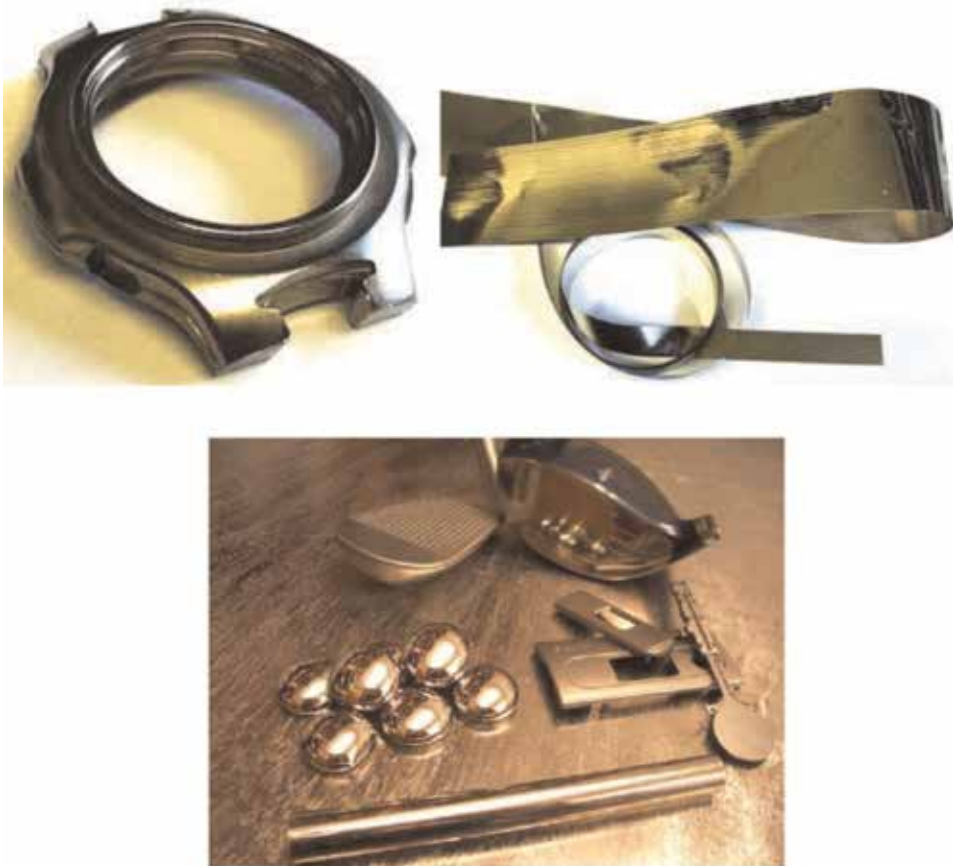
Figure 6. BMG articles fabricated by direct casting method.
