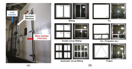
Figure 6. Equipment of the window thermal performance test (a) and shapes of various window types (b).
