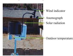
Figure 8. Meteorological data measurement.
