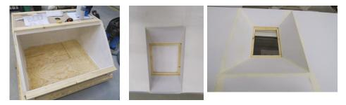
Figure 8. Model of a room for daylight measurement with changeable pitched roof.
