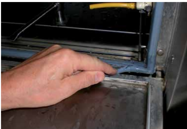
Fig. 4. Damaged rubber gasket in a poorly maintained disinfecter used for reprocessing endoscopes. Formation of biofilm in the disinfecter resulted in a pseudo-outbreak of Mycobacterium gordonae among patients undergoing bronchoscopy with bronchoscopes reprocessed in the disinfecter (Courtesy: Infection Control Team, Odense University Hospital).
