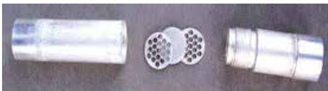
Figure 17. Ag tube, a pressed pellet (diameter 13 mm), and two silver nets for supporting the pellet in the tube and improve the thermal contact during the temperature dependent infrared (TIR) measurements.
