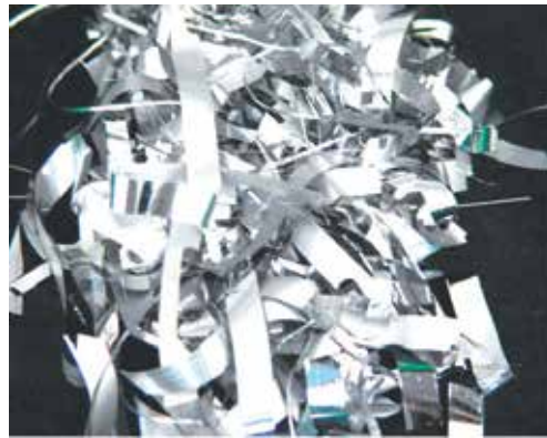
Figure 1. Actual picture of the as-spun (20 m/s) La 2 alloy
