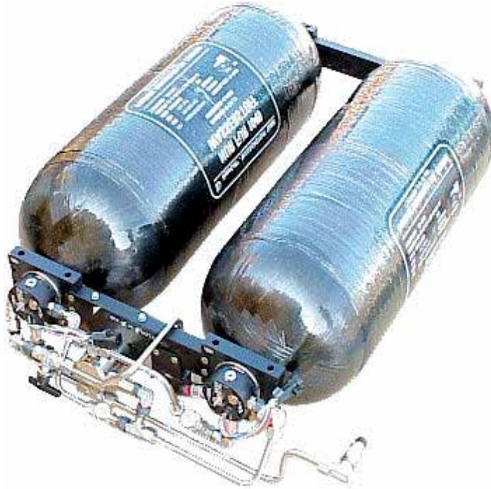
Figure 2. Hydrogen storage in tanks presently used in hydrogen-powered vehicles [12].
