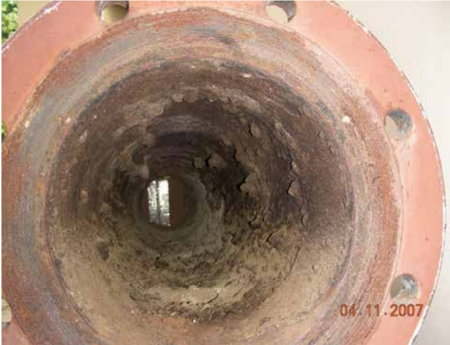
Figure 2. Photography showing the fouling layer formed in a duct section that transports crude oil (Petrobras-BR)
