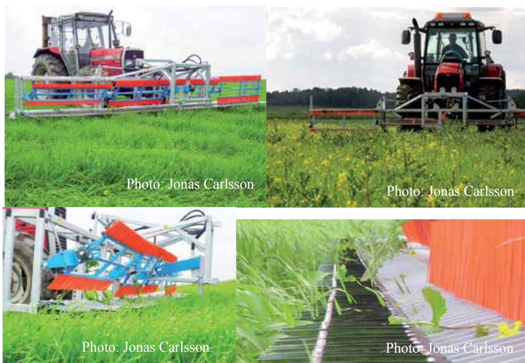
Fig. 7. Weed mower CombCut (upper left and right). Close up pictures of the brush reel (lower left) and the knives (lower right). Photo: Jonas Carlsson, JustCommonSense AB.
