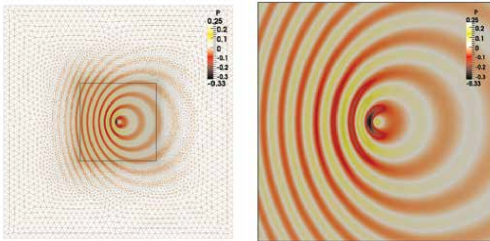
Fig. 17. Convected monopole - M=0.5 , 200 \times 200 grid, t = 270 at y = 0
