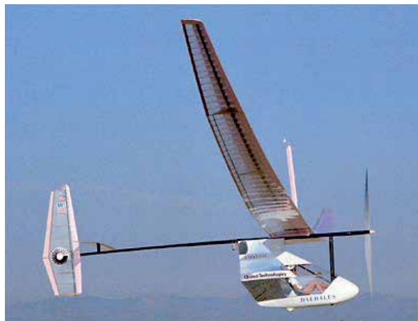
Fig. 3. Daedalus human-powered aircraft (Massachusetts Institute of Technology, Photo/NASA/Beasley)
