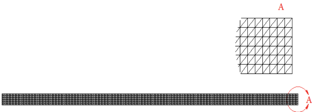
Fig. 4. Mesh for two-dimensional simulations.
