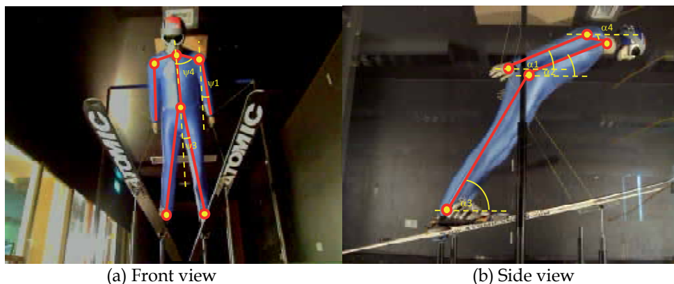
Fig. 3. Angles of different body parts of a ski jumper
