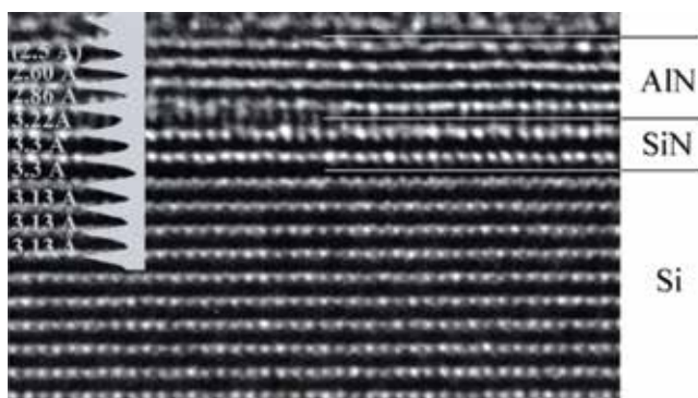
Figure 7. HRTEM image of layers of SiN and AlN on the Si (111) surface.
