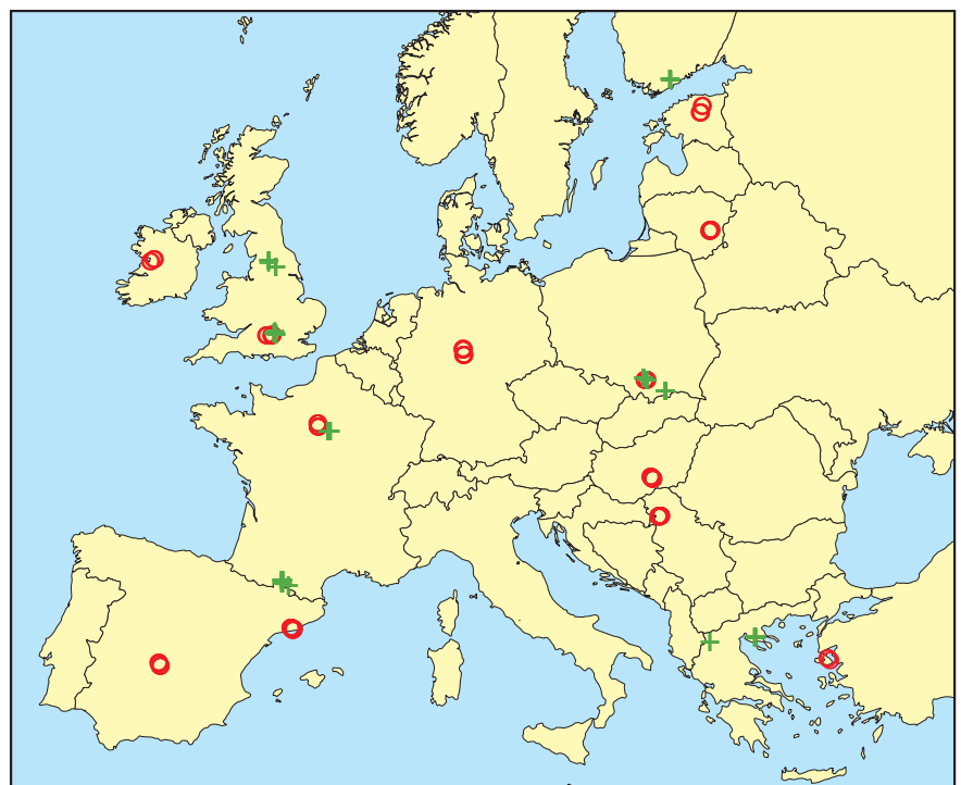
Figure 3. Locations of temperature sensors yielding data used to fit the microclimate models (green crosses) and of those yielding data used to test the models (red circles).
