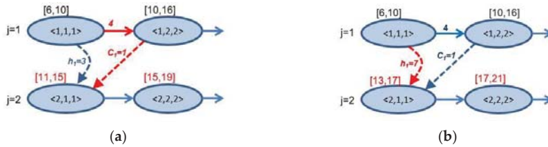
Figure 3. Adding the clear time and headway time distance to the alternative graph: (a) the starting time of operation o_{2,1} is increased due to the clear time; (b) the starting time of operation o_{2,1} is increased due to the headway distance.
