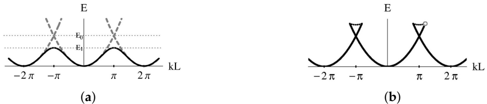
Figure 3. (a) The dashed line schematically shows the energy dispersion for a free particle which is modified to the solid line showing the (lowest) band structure on the application of a periodic potential of period L . (b) Schematic plot of energy bands for a superfluid in an optical lattice that screens out the lattice to maintain non-zero flow velocity at the zone edge. Plots taken from [35].
