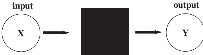
FIGURE 1.5: Illustration of the black box. A set of inputs and outputs determines the object without any study of the interior structure.
