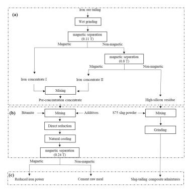
**Figure 2.** Experimental flowsheet: (**a**) The process of pre-concentration; (**b**) the process of iron recovery; (**c**) final products.
