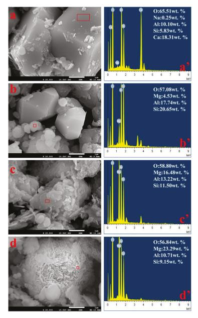
Figure 9. Morphologies of the solid products at 200 °C: (a-a') 0% MgO addition; (b-b') 30% MgO addition; (c-c') 70% MgO addition and (d-d') 100% MgO addition.
