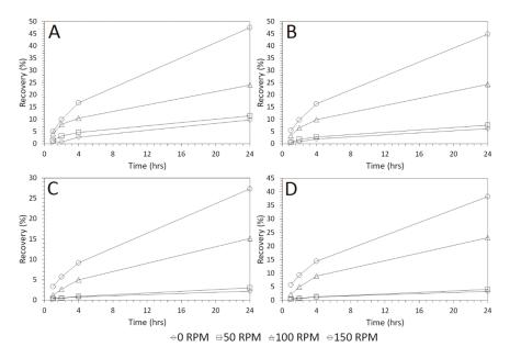
**Figure 11.** As recovery as a function of time for mixing speeds of 0, 50, 100, and 150 RPM using:  $H_2SO_4$  (**A**), HCl (**B**),  $C_6H_8O_7$  (**C**) and  $CH_3SO_3H$  (**D**). The acid concentrations were 1 M and the lixiviant volumes were 200 mL.
