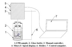
Figure 4. High-shearing-type mixer.
