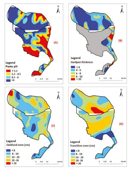
Figure 8. Mapping of: (A) paste pH, (B) hardpan thickness, (C) oxidized zone, and (D) transition zone.
