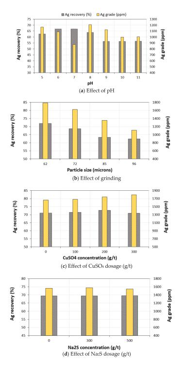
Figure 11. Evolution of silver grade and recovery as a function of: (a) pH; (b) grain size fraction (D90); (c)  $CuSO_4$  dosage (g/t) and (d)  $Na_2S$  dosage (g/t).
