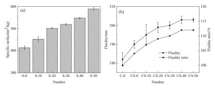
**Figure 6.** Specific surface area and workability of the slag-tailing: (a) Specific surface area when ground for 30 min; (b) fluidity and fluidity ratio of mortars.
