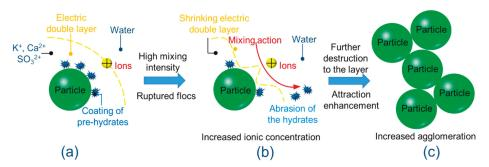
Figure 11. Schematic of the mechanism depicting how high-intensity mixing can lead to increased agglomeration. (a) Electric double layer of particle. (b) Shrinking electric double layer. (c) Particle aggregation.
