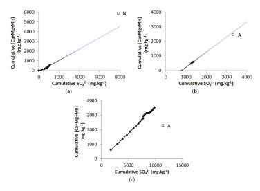
**Figure 7.** Extrapolation of the oxidation-neutralization curves and projection of the samples initial compositions for (**a**) Kittilä, (**b**) Meliadine, and (**c**) Westwood. A: acid-generating samples; N: neutralizing samples.
