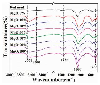
Figure 8. FTIR spectra of solid samples at 200 °C.
