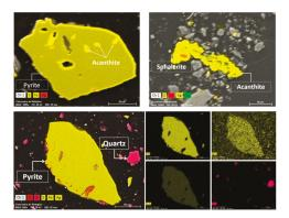
Figure 13. Combined BSE SEM and X-mapping images of the main silver bearing minerals.
