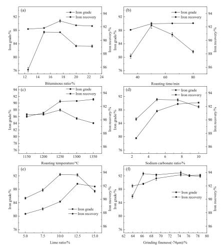
Figure 3. Effect of different influencing factors on iron recovery and iron grade: (a) Bituminous ratio; (b) roasting time; (c) roasting temperature; (d) sodium carbonate ratio; (e) lime ratio; (f) grinding fineness.
