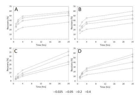
**Figure 9.** As recovery as a function of time for solid–liquid ratios of 0.025, 0.05, 0.2, and 0.4 using:  $H_2SO_4$  (**A**), HCl (**B**),  $C_6H_8O_7$  (**C**) and  $CH_3SO_3H$  (**D**). The acid concentrations were 1 M and the lixiviant volumes were 200 mL.
