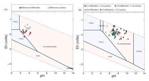
Figure 9. Fe and S pH–Eh diagrams for the leachates from (A) the reference cell and (B) amended tailings.
