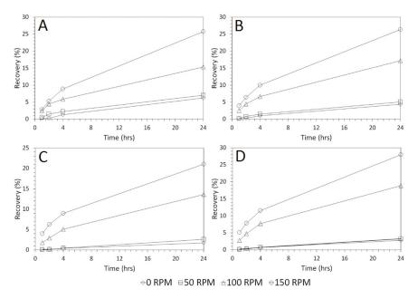
**Figure 10.** Cu recovery as a function of time for mixing speeds of 0, 50, 100, and 150 RPM using:  $H_2SO_4$  (**A**), HCl (**B**),  $C_6H_8O_7$  (**C**) and  $CH_3SO_3H$  (**D**). The acid concentrations were 1 M and the lixiviant volumes were 200 mL.
