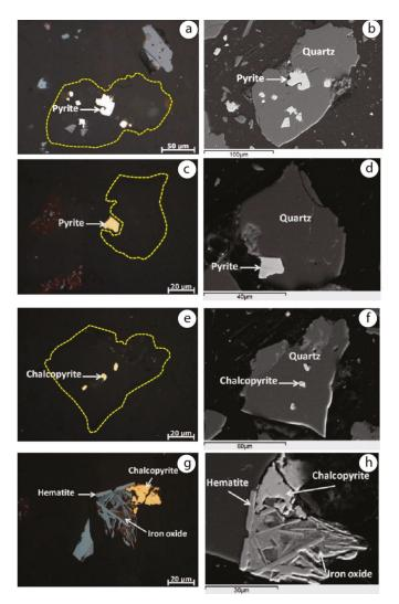
Figure 6. The identified sulfide minerals within the desulfurized tailings obtained from the flotation test; optical microscopy (a,c,e,g) and SEM (b,d,f,h).
