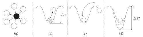
**Figure 9.** A simple illustration of the thixotropic behavior of CPB. (a) The particle interaction forces determine for each particle a potential energy well. (b) The particle does not leave the well. (c) The particle has the ability to get out of the well. (d) The potential energy well tends to be deeper at rest with time, the particle needs a larger amount of energy to get out of the well.
