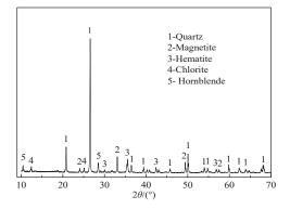
Figure 1. XRD pattern of the IOTs.
