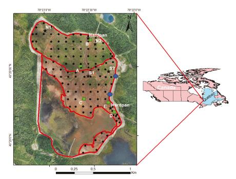
Figure 2. Map showing the sampling grid at the Joutel mine site. N1, N2, S1, and S2 refer to oxygen consumption test locations done on tailings, hardpan (north) and hardpan (south) correspond to oxygen consumption tests done on hardpan, and the green tiles correspond to samples analyzed using QEMSCAN. Red polygon corresponds to the TSF dam and blue circles correspond to the input locations of tailings.
