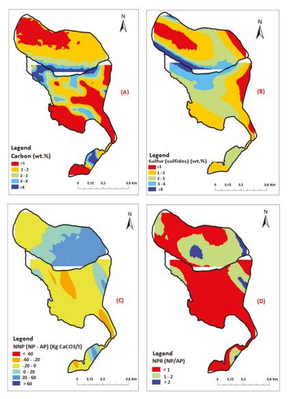
Figure 9. Results of the mapping of: (A) C<sub>inorganic</sub> (B) S<sub>sulfide</sub>, (C) NNP, and (D) NPR.
