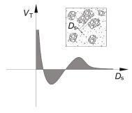
**Figure 1.** Total potential energy interaction  $V_{\rm T}$  between particles.
