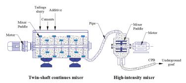
Figure 2. The high-intensity mixing technology of cemented paste backfill (CPB).
