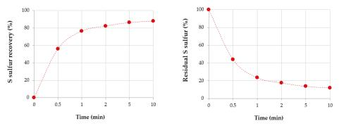
Figure 4. Flotation kinetic of the tailing: (a) % of S<sub>sulfide</sub> recovery vs. time; (b) residual % S<sub>sulfur</sub> vs. time.
