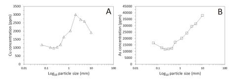
Figure 4. Cu (A) and As (B) concentrations as a function of particle size.
