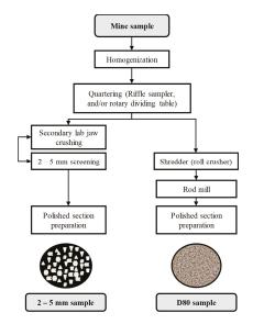
Figure 1. Lab preparation procedure to obtain the two different polished sections.
