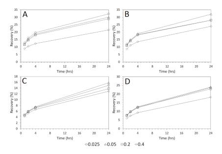
**Figure 8.** Cu recovery as a function of time for solid–liquid ratios of 0.025, 0.05, 0.2, and 0.4 using:  $H_2SO_4$  (**A**), HCl (**B**),  $C_6H_8O_7$  (**C**) and  $CH_3SO_3H$  (**D**). The acid concentrations were 1 M and lixiviant volumes were 200 mL.
