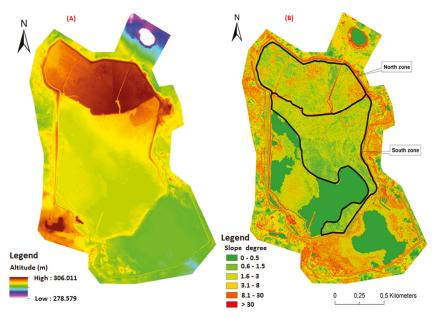
Figure 7. (A) Digital elevation model and (B) slope map within the Joutel TSF.
