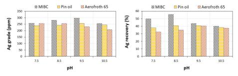
Figure 9. Grade and recovery of silver for different types of frothers and under different pH levels.
