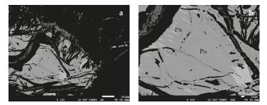
**Figure 3.** (a) Flames of pentlandite in a pyrrhotite grain, Raglan sample; (b) Zoom on the flames of pentlandite (Pn) in pyrrhotite (Po).
