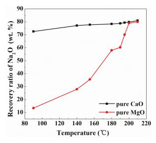
Figure 3. Influence of temperature on the recovery ratio of Na<sub>2</sub>O using pure CaO/MgO (t = 3 h).
