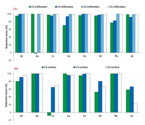
**Figure 10.** Reduction factors for Al, As, Cr, Cu, Fe, Ni, Pb, and Zn for the different amendment formulations. (**A**) Vertical infiltration leachates; (**B**) surface and subsurface runoff leachates.
