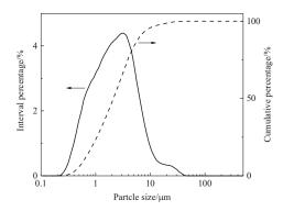
Figure 8. Particle size distribution curve for the slag-tailing admixtures of CS-20.
