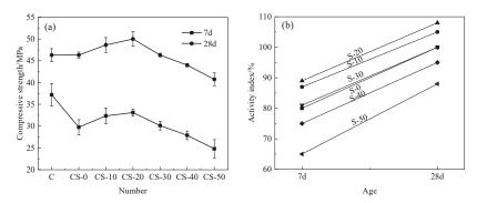
Figure 7. Compressive strength of mortars and activity index of slag-tailing admixture: (a) Compressive strength of mortars; (b) activity index of slag-tailing admixture.
