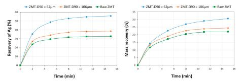
Figure 7. Flotation kinetics of mineral silver at two grain sizes: (a) silver recovery and (b) mass recovery as a function of flotation residence time.
