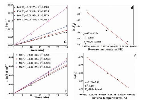
**Figure 7.** Kinetic fitting of (a) the plots of  $[1 - \frac{2}{3}\alpha (1 - \alpha)^{2/3}]$  versus time for CaO, (b)  $\ln(K_a)$  versus temperature for CaO, (c) the plots of  $[1 - (1 - \alpha)^{1/3}]$  versus time for MgO lower than 200 °C, (d)  $\ln(K_a)$  versus temperature for MgO lower than 200 °C, (e) the plots of  $[1 - \frac{2}{3}\alpha - (1 - \alpha)^{2/3}]$  versus time for MgO higher than 200 °C and (f)  $\ln(K_a)$  versus temperature for MgO higher than 200 °C.
