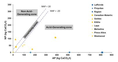
**Figure 6.** Net neutralization potential values for the ten ore samples calculated from the neutralization potential (NP) by Plante [52] and from the acid-generation potential (AP) by Chopard et al. [54].
