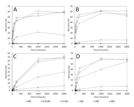
**Figure 7.** As recovery as a function of time for each acid concentration for each acid type:  $H_2SO_4$  (**A**), HCl (**B**),  $C_6H_8O_7$  (**C**) and  $CH_3SO_3H$  (**D**). A solid–liquid ratio of 0.1 and lixiviant volume of 200 mL were used for each experiment.
