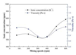
Figure 10. Relationship between ionic concentration (K<sup>+</sup>) and viscosity of CPB-D.
