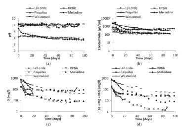
**Figure 4.** Geochemical results from the weathering cells: (a) pH and (b) electrical conductivity; (c,d) concentrations (mg/L) of metals associated with sulfide oxidation in the ore samples: (c) S, (d) Ca + Mg + Mn.
