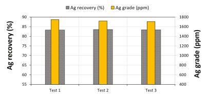
Figure 12. Silver recovery and grade under the optimized conditions.
