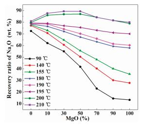
**Figure 4.** Influence of blending MgO and CaO on the recovery ratio of Na<sub>2</sub>O (t = 3 h, % means the mole fraction of MgO addition).
