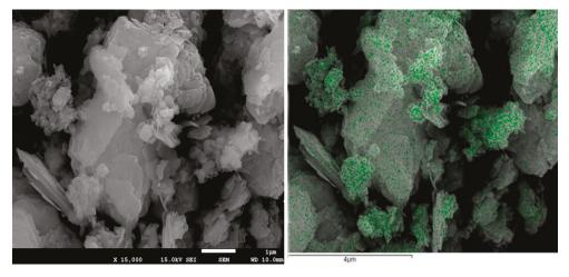
Figure 2. Morphology of the red mud (the green parts represent Na).
