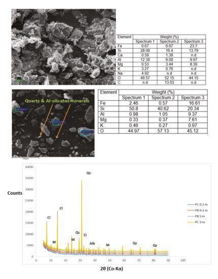
**Figure 4.** Representative scanning electron microscopy-energy dispersive spectroscopy (SEM-EDS) under 10 and 100 µm magnification and X-ray diffraction (XRD) patterns within tailings profile C at a depth of 2.5 m. Abbreviations: Qz—quartz, Cl—clinochlore, M—muscovite, Alb—albite, n.d—not detected.
