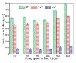
Figure 6. Results of the inductively coupled plasma mass spectrometry (ICP) test for CPB-D.
