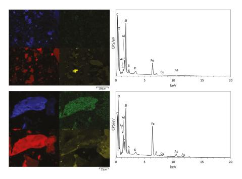
**Figure 2.** SEM-EDX maps for As (blue), Cu (green), Fe (yellow), and S (red) for the mine tailings along with corresponding spectra for CPS/eV detected for each element within the detection range of 0–20 keV.
