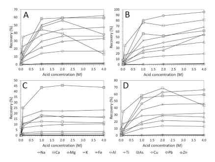
**Figure 5.** Metal recovery as a function of acid concentration after 48 h for each acid type:  $H_2SO_4$  (**A**), HCl (**B**),  $C_6H_8O_7$  (**C**) and  $CH_3SO_3H$  (**D**) A solid–liquid ratio of 0.1 and lixiviant volume of 200 mL were used for each experiment.
