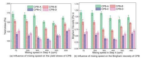
Figure 8. Influence of mixing speed on the yield stress (a) and Bingham viscosity (b) of CPB.
