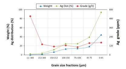
Figure 6. Distributions and grades of silver in different grain size fractions.
