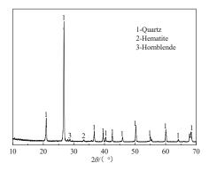
Figure 5. XRD pattern of the high-silica residues.
