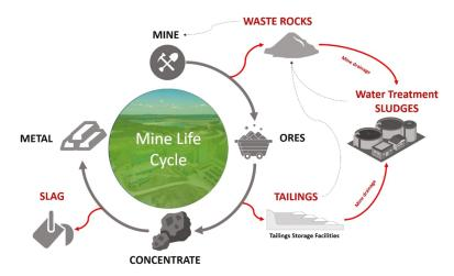
Figure 1. A mine's life cycle and types of mine wastes.
