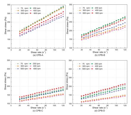
**Figure 7.** Influence of mixing speed on flow curve behaviors depending on different CPBs: (a) CPB-A; (b) CPB-B; (c) CPB-C; and (d) CPB-D.
