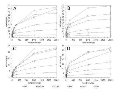
**Figure 6.** Cu recovery as a function of time and acid concentration for:  $H_2SO_4$  (**A**), HCl (**B**),  $C_6H_8O_7$  (**C**) and CH<sub>3</sub>SO<sub>3</sub>H (**D**). A solid–liquid ratio of 0.1 and lixiviant volume of 200 mL were used for each experiment.
