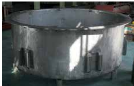
Fig. 20. Image of the manufactured CSB mockup
