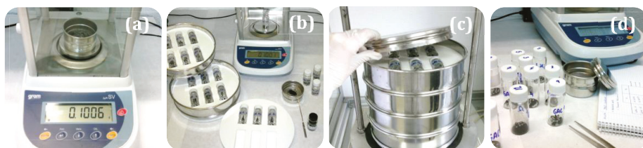
Figure 2. Depiction of materials and procedure for the mechanical strength evaluation of the samples: (a) a weighted sample was sieved using in 300 \mu m sieve and put in a vial; (b) 15 steel balls were also incorporated in the vial, which was then placed in a polymer mold; (c) the molds were placed in the sieve shaker during 20 min; (d) the sample was sieved again in a 300 \mu m sieve and the residue (the sample not converted to dust in the sieving step) was collected and weighed to calculate the sample remaining mass percentage (SRM%).
