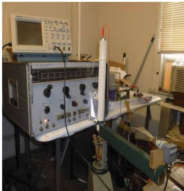
Figure 7. Plasma beam steering experiment. Antenna rotator with holder (green) and receiver horn/detector is in the foreground. The oscilloscope used to monitor the signal waveform is on top of the HP signal generator. The solid state pulsing circuit is to the right of the signal generator.
