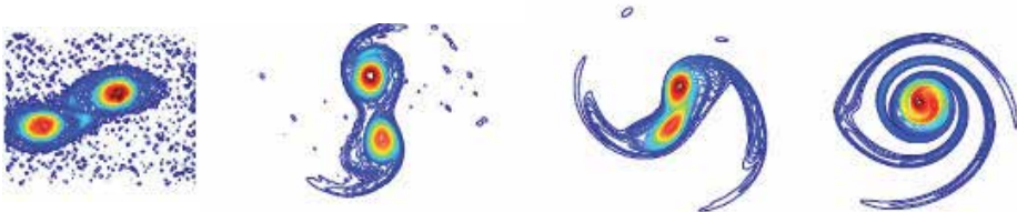
Fig. 12. PIV of vorticity distribution of leapfrogging vortex rings in the symmetry plane of a high Reynolds number jet obtained with a moving window technique by Bricteux et al 2011.
