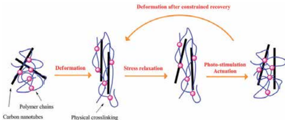
Figure 1. Principle of photo-actuation behavior of physically or chemically cross-linked systems.
