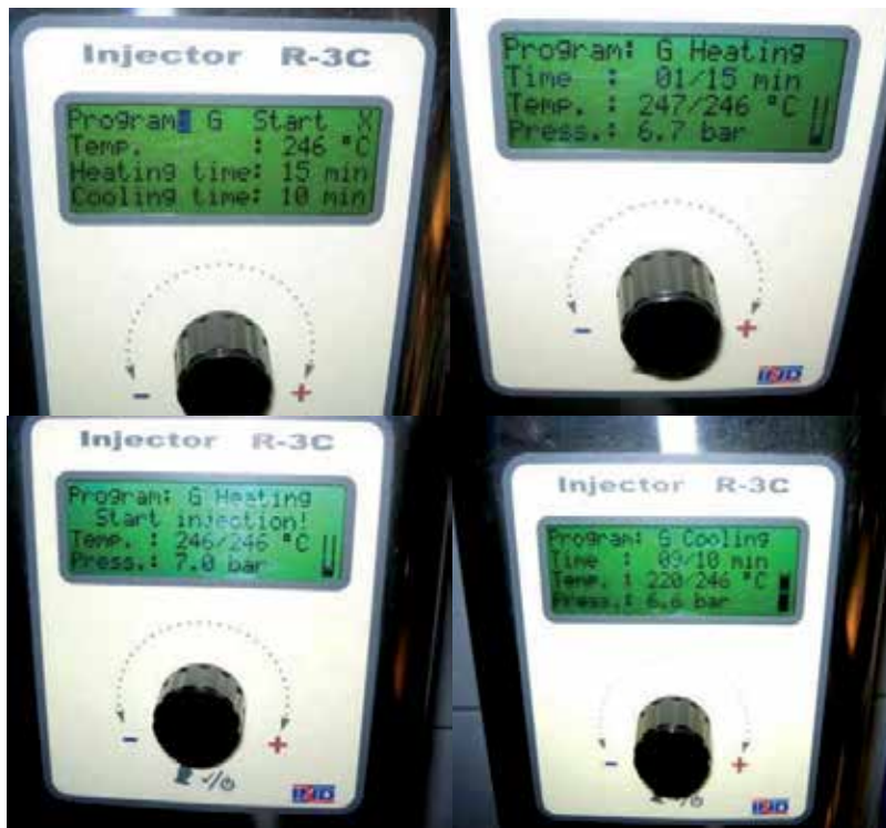
Figure 12. Schedule of "G" program of injecting the thermoplastic material (a) Start (b) Heating (c) Injecting (d) Cooling
