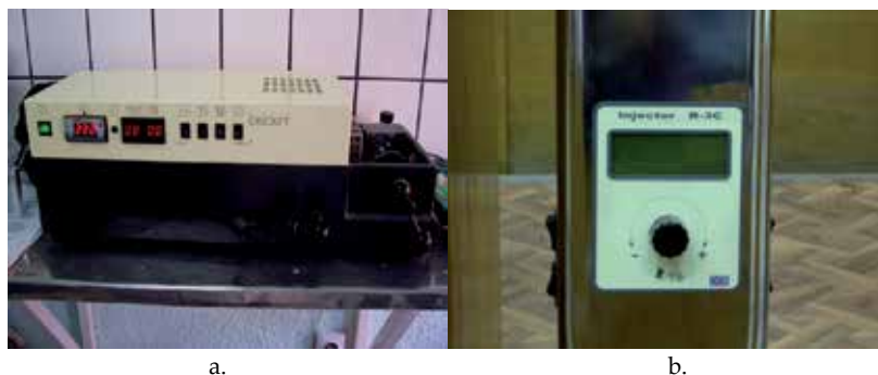
Figure 4. (a) The Polyapress injection-molding device (Bredent) (b) The R-3C injector (Flexite)
