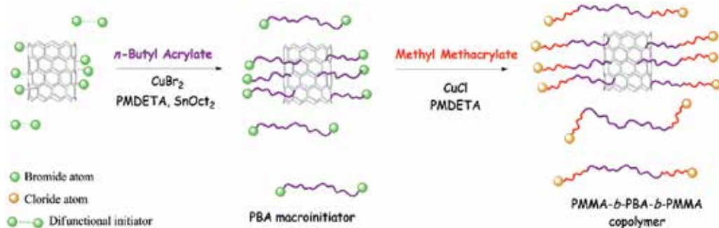
Figure 14. Schematic illustration of covalent modification of MWCNT surface with PBA- b -PMMA diblock copolymer in situ during synthesis of PMMA- b -PBA- b -PMMA matrix [48].
