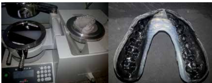
Figure 25. Laminating the custom-made mouth guard. Custom made mouth guard
