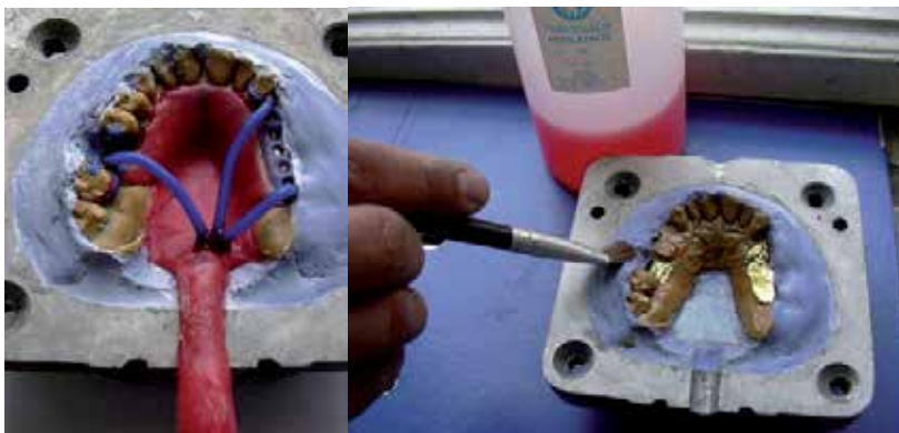
Figure 11. (a) Wrapping the wax pattern frame of the removable partial denture (b) Insulation of the investment
