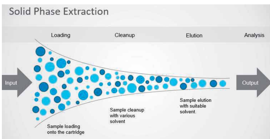
Figure 6. Solid phase extraction technique.
