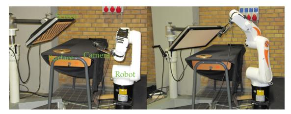
**Figure 6.9:** Photo of the experimental setup. The left picture shows the first step: the determination of the screen position. The right picture is taken while the deflectometric measurement is acquired.
