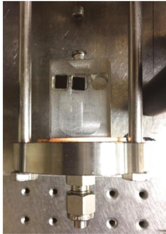
**Figure A7.** Custom designed sample holder. The block copolymer film sits in the center well, a silicon optical standard sits in the left well. A hole for background ultraviolet-visible (UV-V) light is spectroscopy subtraction is on the right. The sample holder rests on a two-pronged frame to slide the samples in and out of the main chamber and is sealed with a Conflat flange with copper gasket.
