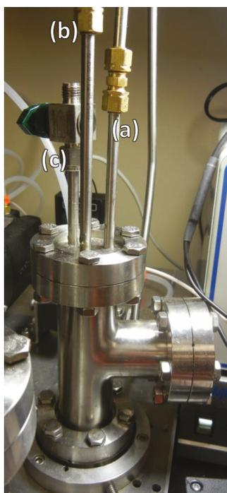
**Figure A6.** Depiction of the solvent reservoir with three  $\frac{1}{4}$ " tubing ports. One tube (a) is an  $N_2$  inlet that extends to the bottom of the reservoir. One tube (b) is a solvent vapor outlet that only extends into the reservoir  $\frac{1}{2}$ " to capture the vapor. One tube (c) is capped with a normally-closed plug valve. This is used to add liquid solvent without opening the Conflat flanges.
