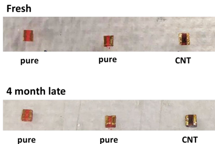
Figure S1. The stability of carbon-in-perovskite and pure perovskite single crystals-based photodetectors.
