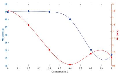
Figure 7. Saturation magnetization and coercive field versus Ti concentration.
