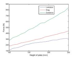
Figure 16. Levitation force as a function of plate height.
