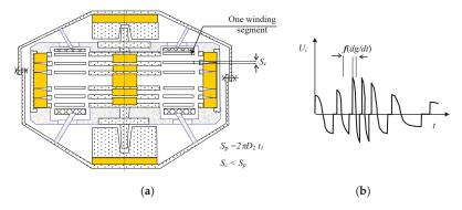
**Figure 11.** A component diagram of the MG0 design with the linearized coefficient of stiffness *k* (based on principle II); (**a**) configuration B, and (**b**) its output voltage.
