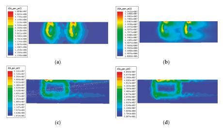
**Figure 9.** Distribution of eddy currents on plate surface at different speeds with single magnet, (**a**) 2 m/s, (**b**) 10 m/s, (**c**) 70 m/s, and (**d**) 100 m/s.
