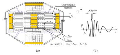
**Figure 12.** A component diagram of the MG0 design with the linearized coefficient of stiffness *k* (based on principle II); (**a**) configuration C, and (**b**) its output voltage.
