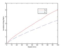
Figure 8. Levitation drag ratio over magnet velocity.
