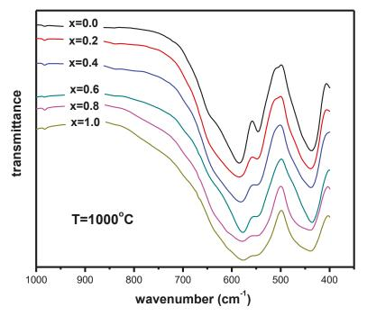
**Figure 4.** IR spectra of  $BaFe_{12-x}Ti_xO_{19}$  sintered at T = 1000 °C.
