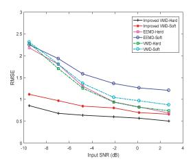
**Figure 8.** The root-mean-square deviation (RMSE) of the EEMD, the VMD, and the improved VMD methods are revealed, for both soft and hard thresholding of interval thresholding. The improved VMD method outperforms other methods.
