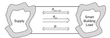
Figure 4. Flux of the generalized Poynting multivector components of electrical systems.
