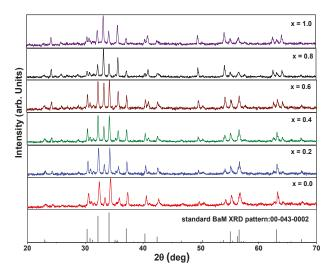
**Figure 2.** XRD patterns  $BaFe_{12-x}Ti_xO_{19}$  samples with (x = 0.0-1.0) sintered at 1000 °C for 1 h and shown the standard XRD pattern of  $BaFe_{12}O_{19}$  (file no.: 043-0002).
