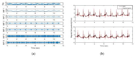
**Figure 5.** The noisy signal and the IMFs obtained from VMD are shown in (**a**). A comparison of the original signal (dotted line) with the reconstructed signals (solid line) obtained from VMD based denoising methods with soft and hard thresholding is shown in (**b**). The panel above is the result of hard thresholding processing and the following panel is the result of soft thresholding processing.
