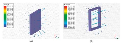
Figure 11. Rainbows of magnetic field vector, (a) PM, (b) SC magnet.
