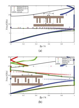
**Figure 5.** Brillouin diagram of a parallel-plate waveguide with periodic metallic corrugations (a) symmetrically and (b) non-symmetrically distributed. Short period: p = 6 mm. Other parameters: h = 10 mm, s = 2 mm, t = 1 mm and g = 1 mm.
