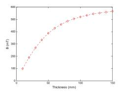
Figure 13. Magnetic flux density over magnet thickness.
