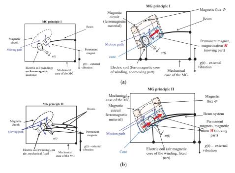
**Figure 1.** The principal configuration of the core of the milli- or micro generator (MG): (**a**) a beam version, principle I; (**b**) a beam version, principle II [2].
