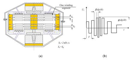
**Figure 10.** A component diagram of the MG0 design with the linearized coefficient of stiffness k (based on principle II); (a) configuration A, and (b) its output voltage  $U_{out}$ .
