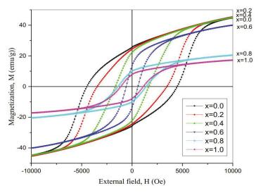
**Figure 6.** Hysteresis loops for the samples  $BaFe_{12-x}Ti_xO_{19}$  (x = 0.0 - 1.0) sintered at 1000 °C.
