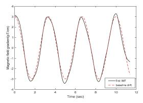
**Figure 6.** The first IMF obtained from the improved VMD method (solid line) and baseline drift noise (dotted line). It is seen that the solid line and the dotted line basically coincide. This method can effectively remove baseline drift noise.
