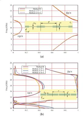
**Figure 3.** Dispersion diagram of the periodic printed microstrip lines shown as insets. The substrate of the lines has thickness *h* and relative permittivity  $\varepsilon_r$ . (**a**) p = 5.6 mm, w = 0.6 mm,  $w_s = 0.2$  mm,  $\varepsilon_r = 10.2$  and h = 0.635 mm; (**b**) p = 4 mm, w = 0.6 mm, g = 0.2 mm,  $\varepsilon_r = 10.2$  and h = 0.767 mm.
