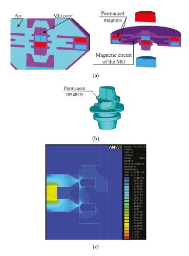
**Figure 6.** A geometrical rotationally SYMMETRIC model of the MG0 based on principle II [2]: (**a**) the ANSYS geometrical model; (**b**) the core; and, (**c**) the optimal design, detailed distribution of the magnetic flux density module *B* [T].
