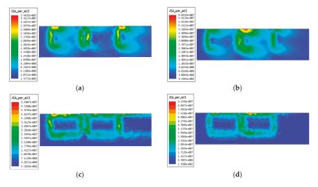
**Figure 15.** Distribution of eddy currents on plate surface at different speeds with NN and NS arranged magnets: (**a**) NN magnets at 10 m/s, (**b**) NS magnets at 10 m/s, (**c**) NN magnets at 100 m/s, and (**d**) NS magnets at 100 m/s.
