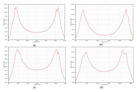
**Figure 12.** Distributions of magnetic flux density: (**a**) Y direction of PM, (**b**) Z direction of PM, (**c**) Y direction of SC magnet, and (**d**) Z direction of SC magnet.
