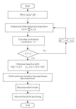
Figure 1. The flow chart of the improved Variational Mode Decomposition (VMD) algorithm.
