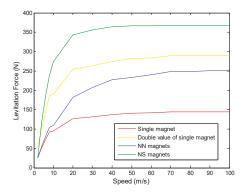
Figure 14. Levitation forces with different magnet arrangements (NN and NS) over magnet velocity.
