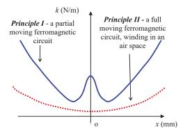
**Figure 8.** The applied stiffness characteristics [2], coefficient *k*; the behavior is nonlinear in both of the MG magnetic circuit principles.
