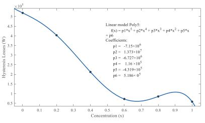
**Figure 9.** Hysteresis losses (in W) BaFe<sub>12-x</sub>Ti<sub>x</sub>O<sub>19</sub> (x = 0.0-1.0) sintered at 1000 °C.
