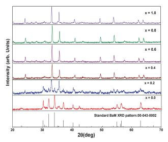
**Figure 1.** XRD patterns for BaFe<sub>12-x</sub>Ti<sub>x</sub>O<sub>19</sub> samples with (x = 0.0-1.0) sintered at 850 °C for 1 h and shown the standard pattern of BaFe<sub>12</sub>O<sub>19</sub> (file no.: 043-0002).
