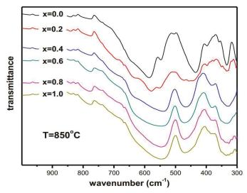
**Figure 3.** Infra-Red (IR) spectra of  $BaFe_{12-x}Ti_xO_{19}$  sintered at T = 850 °C.
