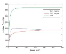
Figure 18. Simulation results of levitation forces of the front and the back magnets.
