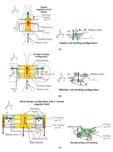
**Figure 2.** The basic arrangement of the investigated rotationally symmetric geometry device exploiting Faraday's induction law: (**a**) the classic solution; (**b**) the novel arrangement; and, (**c**) the option with a closed magnetic circuit to minimize (optimize) the impact of external magnetic fields [2].
