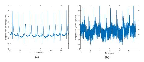
**Figure 2.** A comparison of the approximately pure magnetocardiography (MCG) signal with the noisy signal; waveform characteristics can be clearly seen in (**a**); (**b**) shows the signal waveform with three kinds of noise. The signal is drowned in the noise under high noise circumstances.
