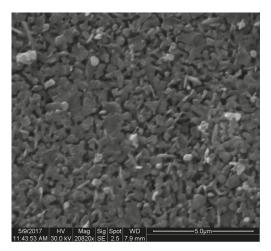
**Figure 5.** SEM image for BaFe<sub>12-x</sub>Ti<sub>x</sub>O<sub>19</sub> (x = 0.2) sample sintered at T = 1000 °C.
