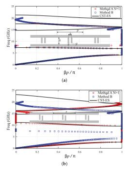
**Figure 4.** Brillouin diagram of a parallel-plate waveguide (PPW) with periodic metallic corrugations (a) symmetrically and (b) non-symmetrically distributed. The inset structures represent longitudinal sections of the PPW's with the grey color standing for the metallic parts of the structures. Long period: p = 12 mm. Other parameters: h = 10 mm, s = 2 mm, t = 1 mm and g = 1 mm.
