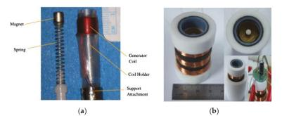
**Figure 18.** The permanent magnet (**a**) having a spring in the cylindrical structure of the energy harvester [18], (**b**) tested sample designed by Lee et al. [17].
