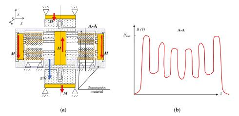
**Figure 3.** The basic arrangement of the investigated device exploiting Faraday's induction law: (**a**) the MG core; and (**b**) the magnetic flux density distribution along the z axis, line A-A.
