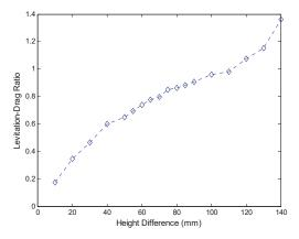
Figure 5. Levitation-drag ratio as a function of height difference h at a speed of 10 m/s.
