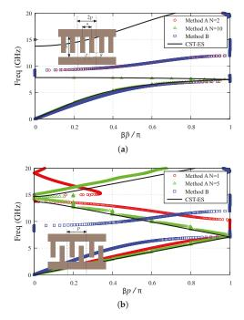
**Figure 6.** Brillouin diagram of a parallel-plate waveguide with periodic metallic corrugations (a) symmetrically  $[\hat{p} = 2p = 4 \text{ mm}]$  and (b) glide-symmetrically distributed [p = 4 mm]. Other parameters: h = 10 mm, s = 2 mm, t = 1 mm and g = 1 mm.
