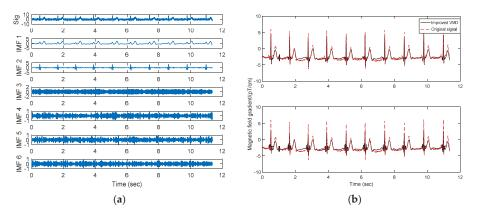
**Figure 7.** (a) The noisy signal and the IMFs obtained from the improved VMD method; (b) A comparison of the original signal (dotted line) with the reconstructed signals (solid line) obtained from the improved VMD method with soft and hard thresholding for interval thresholding. The panel above is the result of hard thresholding processing and the following panel is the result of soft thresholding processing.
