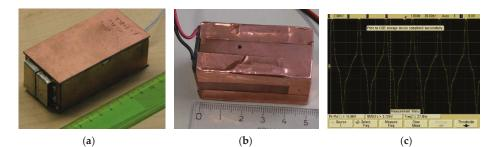
**Figure 20.** The tested microgenerator [2] based on Principle I: (a) MG I—the dimensions of  $90 \times 40 \times 30$  mm,  $U_{\text{out max}} = 300$  V; (b) MG II—the dimensions of  $50 \times 27 \times 25$  mm,  $U_{\text{out max}} = 20$  V; and (c) the instantaneous behavior of the output electrical voltage in MG I and MG II (the effect of the stiffness coefficient *k*—Figure 8).
