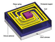
Figure 16. The electromagnetic design by Wang et al. [15].
