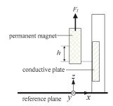
Figure 2. Single plate electrodynamic suspension (EDS) structure.
