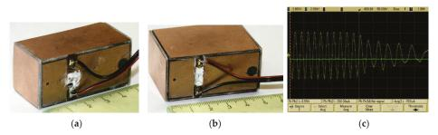
**Figure 21.** The devices based on Principle II [2]: (a) MG III—the dimensions of  $50 \times 25 \times 25$  mm,  $U_{out max} = 10$  V; (b) MG IV—the dimensions of  $50 \times 35 \times 25$  mm,  $U_{out max} = 20$  V; and, (c) the instantaneous behavior of the output electrical voltage in MG III and MG IV (the effect of the stiffness coefficient *k*—Figure 8).
