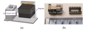
Figure 14. The silicon-based concepts developed by (a) Kulkarni et al. [11] and (b) Zhu et al. [13].
