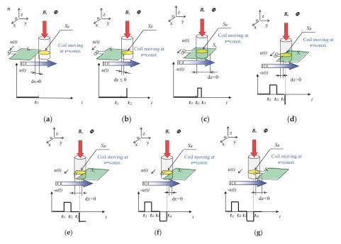
Figure 4. The electric voltage induction in the applied coil, (a-g), according to Faraday's law of induction [2].
