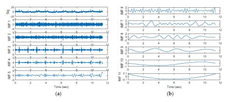
**Figure 3.** The noisy signal and the intrinsic mode functions (IMFs) obtained by Ensemble Empirical Mode Decompositioning (EEMD) are shown in (**a**,**b**).
