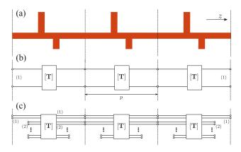
**Figure 1.** Periodic structure under study, period *p*. (a) Cascade of 1-port equivalent networks; (b) Cascade of multi-port equivalent networks; (c) Possible actual appearance of the physical periodic structure with just 3 unit cells.
