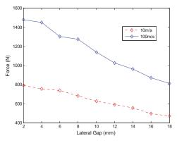
Figure 6. Guidance force as a function of the gap between the magnet and the plate.
