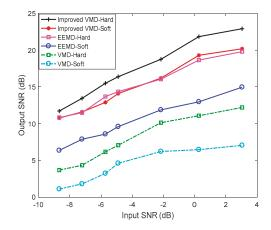
**Figure 9.** The variation of the output signal-to-noise ratio (SNR) by EEMD, VMD and the improved VMD methods with soft and hard thresholds for interval thresholding. The improved VMD method outperforms other methods.
