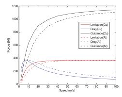
Figure 7. EDS forces as a function of magnet velocity.
