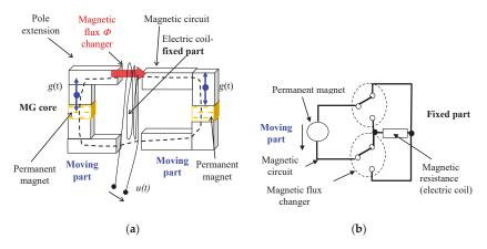
**Figure 7.** The MG core with a ferromagnetic circuit according to principle II [2]: (**a**) a structurally simple variant, acceleration g within the interval of 0.01 g–0.3 g; (**b**) a scheme of the configuration.
