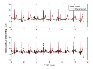
**Figure 4.** A comparison of the original signal (dotted line) with the reconstructed signals (solid line) obtained from EEMD based denoising methods with soft and hard thresholding. The panel above is the result of hard thresholding processing and the following panel is the result of soft thresholding processing.
