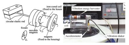
**Figure 17.** The electromagnetic vibration energy harvester using cylindrical geometry, developed by Yang et al. [16].
