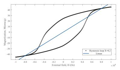
**Figure 8.** The hysteresis loop for the system  $BaFe_{12-x}Ti_xO_{19}$  (x = 0.2) approximated by a straight line.
