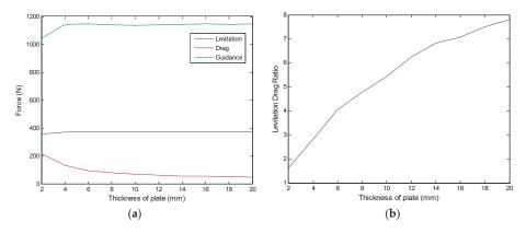
Figure 17. Simulation results of different thicknesses of plate at speed of 100 m/s. (a) Levitation, drag, and guidance forces, (b) levitation drag ratio.
