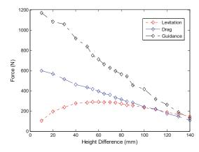
Figure 4. EDS forces as a function of height difference h (speed 10 m/s).
