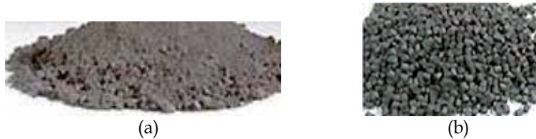
Fig. 3. Mn-Zn ferrite: powder (a) and feedstock (b).
