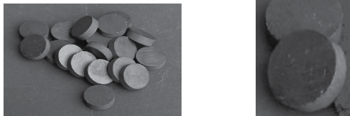
Fig. 4. Disc shaped CIM Mn-Zn ferrite samples (diameter d=16\text{mm} , thickness t=5\text{mm} ).
