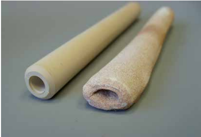
Fig. 10. Comparison of the properly debinded part (left) with the deformed part (right), which was deformed and had granulate wicking agent adhered to the surface. The defect was caused when the part was embedded into a too hot wicking agent, which had not been cooled enough after a thermal regeneration.
