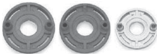
Fig. 2. CIM component: green body, brown body and sintered part, respectively.
