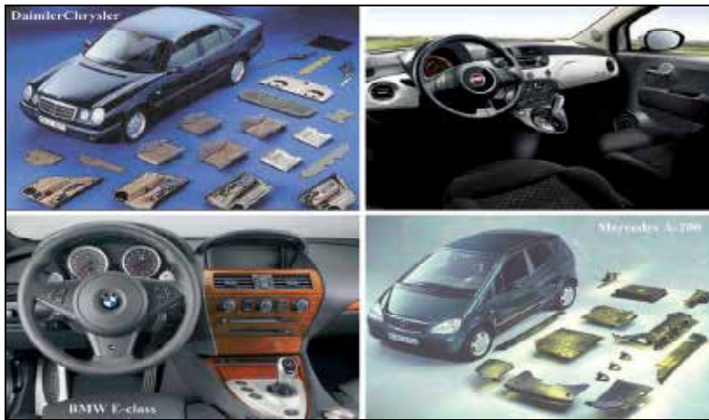
Fig. 3. Some applications of natural fibers in the automotive field.
