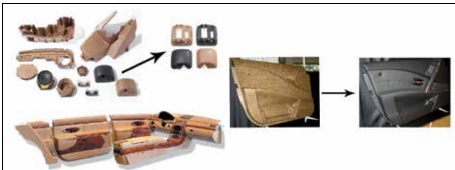
Fig. 4. Interior automotive parts made of wood and natural fiber reinforced plastics.
