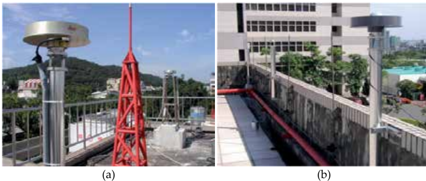
Figure 2. (a) Appearance of fixed stations; (b) Appearance of pillars of calibration base points [1]
