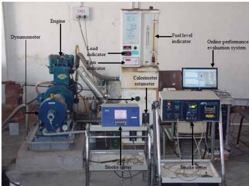
Figure 1. Schematics of the test set-up.
