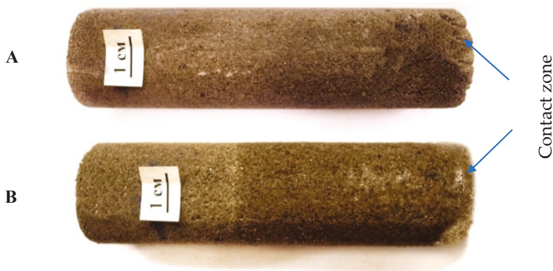
Figure 5. Frozen sandy samples (sand 2, W = 15\% ) before (A) and after interaction (B) with 0.2 N NaCl solution at -3\text{ }^{\circ}\text{C} .
