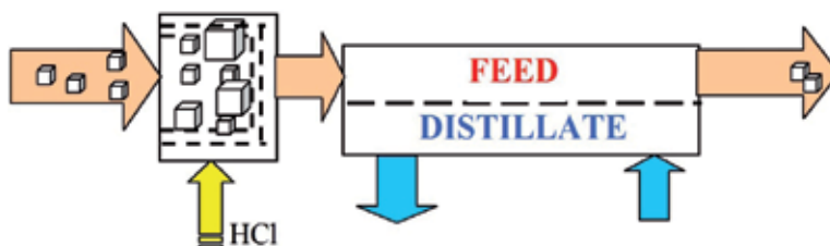
Figure 6. Desalination of effluents using the MD module connected with pre-filtration nets element.
