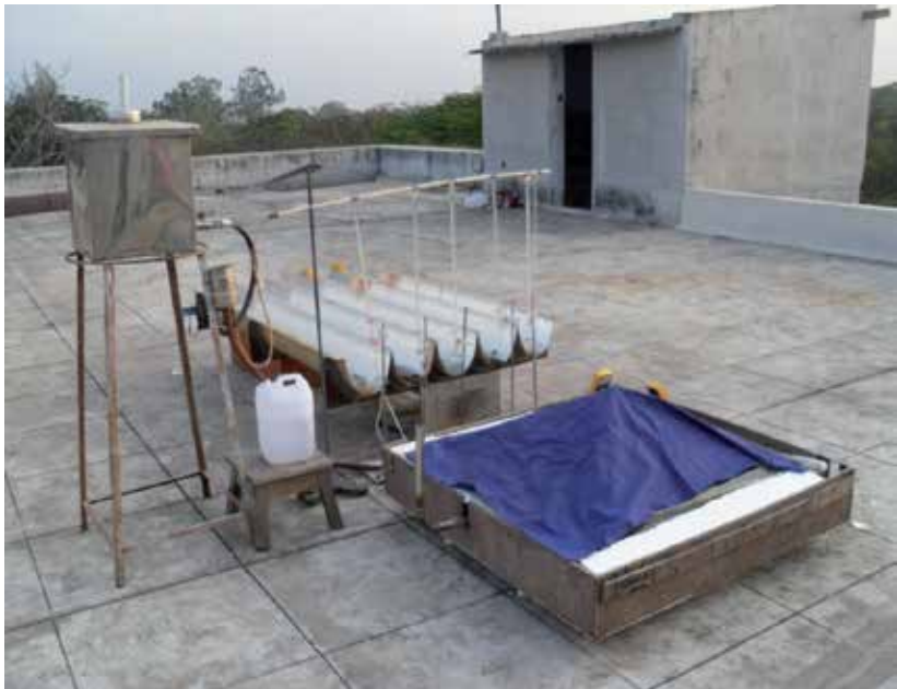
Figure 3. Pictorial view top cover closed pyramid solar still coupled with compound parabolic concentrator tubular solar still.
