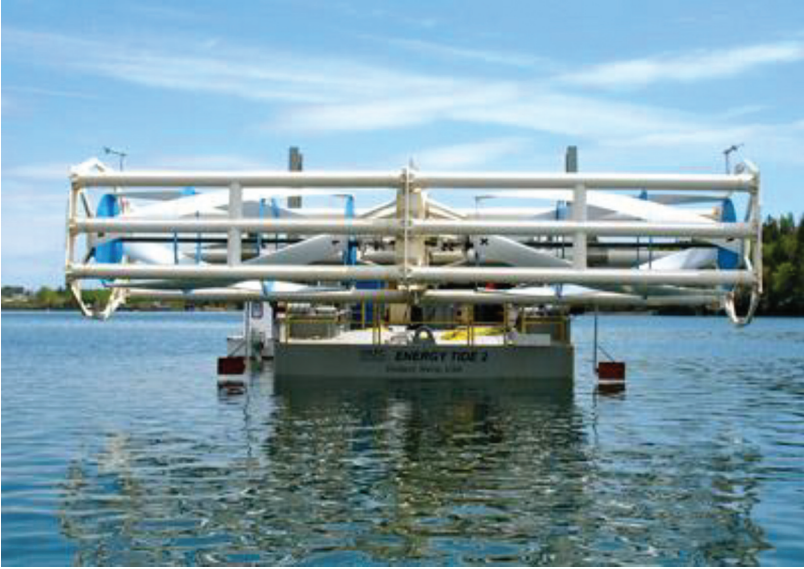
FIGURE 13.6 Cross-flow turbine used in Alaska Rivers: ORPC's TidGen™ power system. [Adapted from “Hydrokinetic energy (in river, tidal, and ocean current),” Alaska Energy Wiki , Alaska Center for Energy and Power, 1–4, 2012.]
