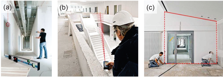
Fig. 1-2: Measurement scenarios. (a) width of hallway, (b) diagonal of staircase (solid red line), (c) length of roof element (photos by courtesy of Robert Bosch GmbH)
