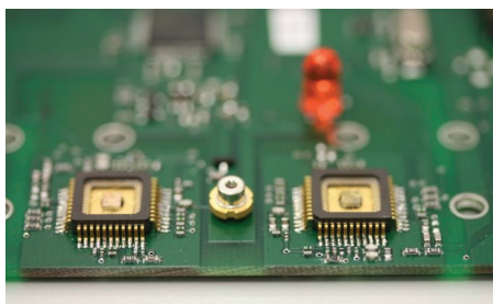
Fig. 6–22: Photograph of two CF340 MPW2011 test chips. The left ASIC modulates the laser (Tx ASIC), the right ASIC acts as the receiver (Rx ASIC) with its laser modulator turned off to prevent crosstalk from laser modulator to binning and SPADs. Both chips are synchronized with a common reference oscillator.
